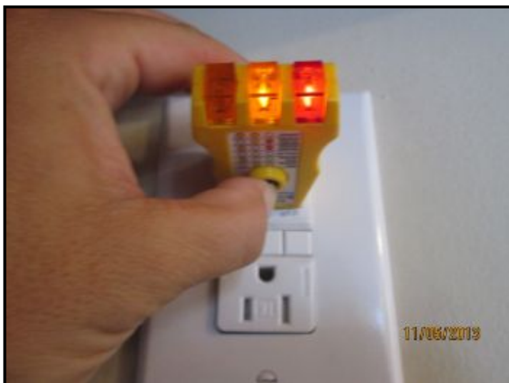
Upside down GFCI and Hot/Neutral Reverse
