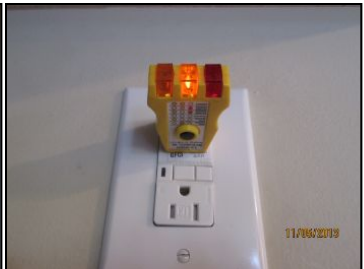
Upside down GFCI and Open ground
